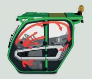
The air conditioning system is completely new and has been developed according to automotive standards, halving the warm-up and cool down times so as to ensure the optimal temperature even in extreme weather conditions. The inlet vent is placed on the side of the cab, away from potential sources of dust and dirt to maximise the service life of the filters. Inside there are eight vents. three of which are dedicated to defrosting the windscreen, for optimal climate comfort.
