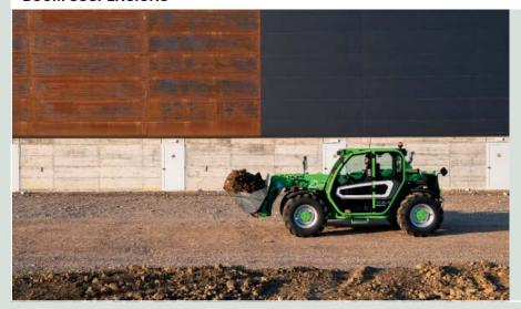
The active boom suspension system (BSS) is available as an option, which protects the load during transfer and maintains a high level of driving comfort on rough terrain. The suspension is automatically deactivated at low speed (below 3 km/h), for boom maximum precision and power.
